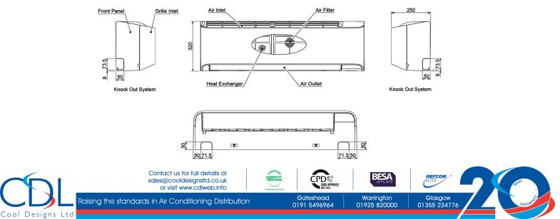
Rated conditions: Cooling : Indoor 27 degC Dry Bulb / 19 degC Wet Bulb , Outdoor 35 degC Dry Bulb. Heating : Indoor 20 degC Dry Bulb , Outdoor 7 degC Dry Bulb / 6 degC WetBulb. Based on equivalent piping length of 7.5m and piping height difference of 0m. Data from Toshiba Air Conditioning 2022
