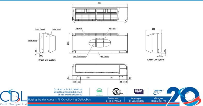
Rated conditions: Cooling : Indoor 27 degC Dry Bulb / 19 degC Wet Bulb , Outdoor 35 degC Dry Bulb. Heating : Indoor 20 degC Dry Bulb , Outdoor 7 degC Dry Bulb / 6 degC WetBulb. Based on equivalent piping length of 7.5m and piping height difference of 0m. Data from Toshiba Air Conditioning 2022
