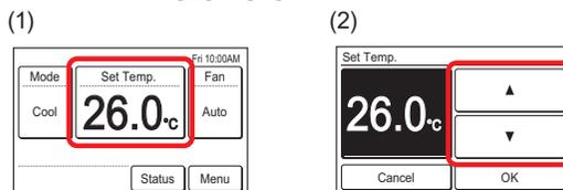
When the operation mode is set to [Custom Auto], set the cooling and heating temperature.
