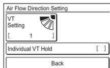
For this operation, refer to “3-2-3 Individual VT Hold”. When the [OK] or [Cancel] is touched at each setting screen, the display returns to this screen. When [Back] is touched, the display returns to the “Main Menu” screen.
