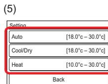
For indoor unit that display [Custom Auto] in the operation mode, set [Cool/Dry] and [Heat]. This setting is reflected in each operation mode of [Custom Auto], [Cool], [Dry] and [Heat].
