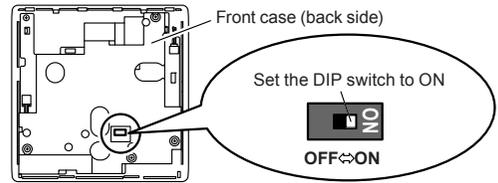
Before using this product, always set DIP switch to "ON". If not set, when the main power is turned on again, the set data by menu operation will be erased and cause erroneous operation.
