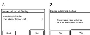
When changing the Master Indoor Unit, another indoor unit cannot be made the master indoor unit unless the settings of the current master indoor unit are cancelled beforehand. ("Reset" cannot be performed while the indoor unit is operating.)
