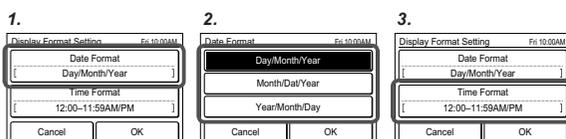
4. Select and touch the data display format. Touch [OK] on the "Time Format" to return to the "Display Format Setting" screen.
