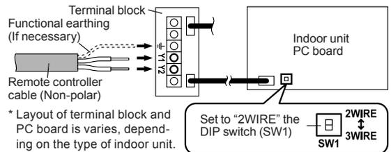
\* Layout of terminal block and PC board is varies, depending on the type of indoor unit.
