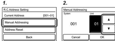
The address for this unit can be set from 1 to 32. However, do not set the same number as that for the remote-control address of an indoor unit connected using the same remote-control cable.
