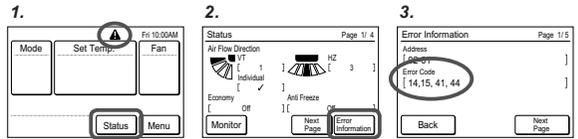
For the details of the indoor unit or outdoor unit error, refer to the error codes in each installation manual.
