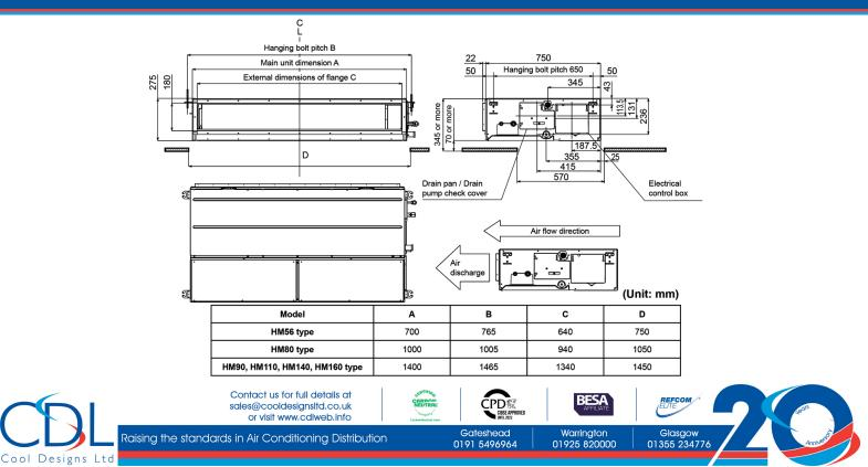
Rated conditions: Cooling : Indoor 27 degC Dry Bulb / 19 degC Wet Bulb , Outdoor 35 degC Dry Bulb . Heating : Indoor 20 degC Dry Bulb , Outdoor 7 degC Dry Bulb / 6 degC WetBulb . Based on equivalent piping length of 7.5m and piping height difference of 0m. Data from Toshiba Air Conditioning 2022
