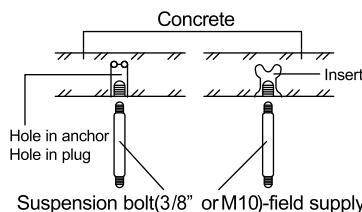
2.2.3 Install the suspension bolts (use W3/8 or M10 suspension bolts, 4 pieces) depending on the ceiling type.
