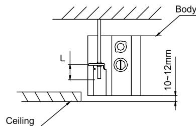
2.3.3 Screw the nuts to suspend the unit. Check the lower side of indoor unit locates at position (10 to 12mm) higher than the lower surface of the ceiling. L is about half of the screw length of the installation hook.
