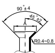
4.1.4 Check if the flaring is properly made. See incorrectly flared pipes sample below.
