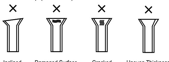
Inclined      Damaged Surface      Cracked      Uneven Thickness
