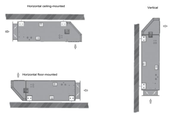
Depending on the type of unit being controlled, it can either be ceiling- or floor-mounted or installed vertically. Ensure a minimum space is left to allow the doors to open (540mm, 595mm, 735mm depending on the configuration). However, if this access cannot be provided, all of the doors can be removed from their hinges to gain access.
