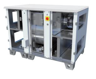
Choose from a selection of heat recovery units to meet your needs: - The plate heat exchanger with the "Classic" model, for all applications where **airtightness** between the flow of fresh air and the flow of extracted air is essential. - The rotary heat exchanger with the "Classic RHE" model, for **optimal heat recovery** all year round and with an optional air circulation function.
