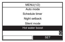
(2) Press the [ ] button to select "ON" on the Hot water boost screen, then press the [ ] button. The mark appears on the top screen.
