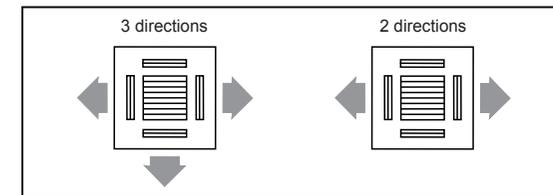
Use a shielding plate kit (sold separately) to change discharge directions. Discharge directions are limited. Follow the Installation Manual supplied with the shielding plate kit.
