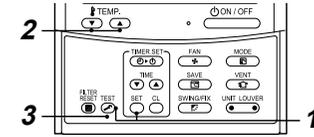
**1** When **SET** and **TEST** buttons are pushed simultaneously for 4 seconds or more, the following display appears.
