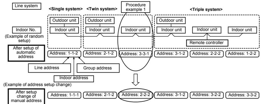
The above address is set by the automatic addressing when the power is turned on. However, line addresses and indoor addresses are set randomly. For this reason, change the setting to match line addresses with indoor addresses.
