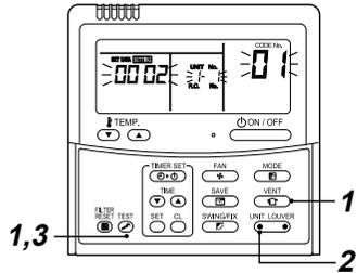
**1 Push TEST + VENT buttons simultaneously for 4 seconds or more.**
