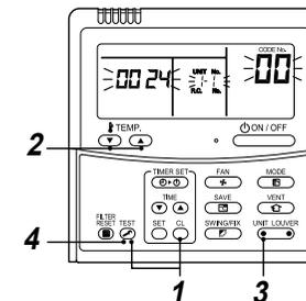
1. Push and buttons simultaneously for at least 4 seconds to call the service monitor mode.
