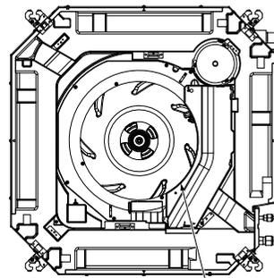
Be sure to remove the tape for transportation between the fan and the bell mouth.
