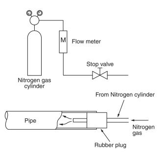
Fig. 6-5-1 Prevention of oxidation during brazing
