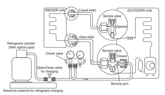
Fig. 6-4-1 Configuration of refrigerant charging
