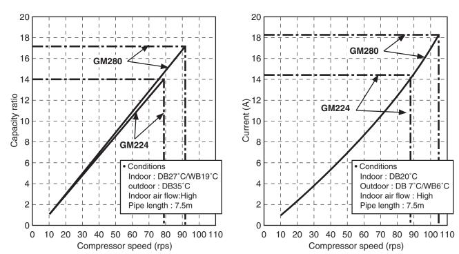
Capacity variation ratio according to temperature
