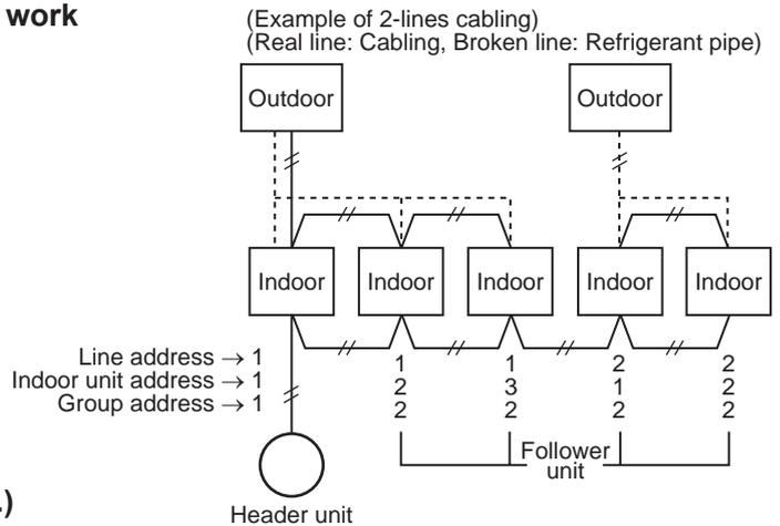
For the above example, perform setting by connecting singly the wired remote controller without remote controller inter-unit cable.
