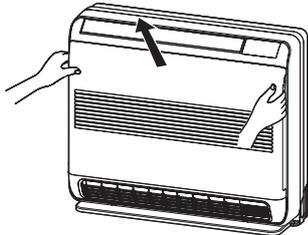
2. Take hold the left and right handles of air filter and push it down to release them from holding slot, then pull it upward to take it out.
