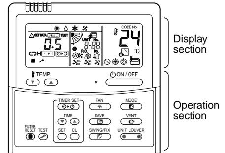
This remote controller can control the operation of Max. 8 indoor units.
