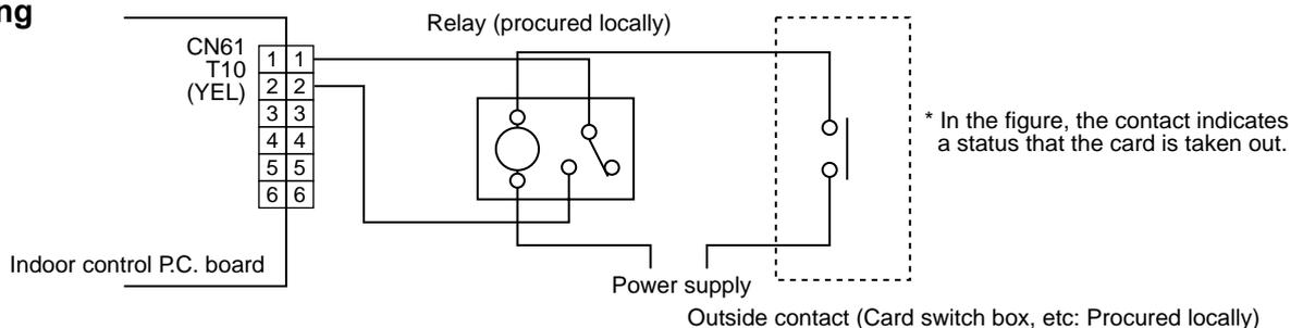
**Note)** Determine the cable length between the indoor control P.C. board and the relay within 2m.
