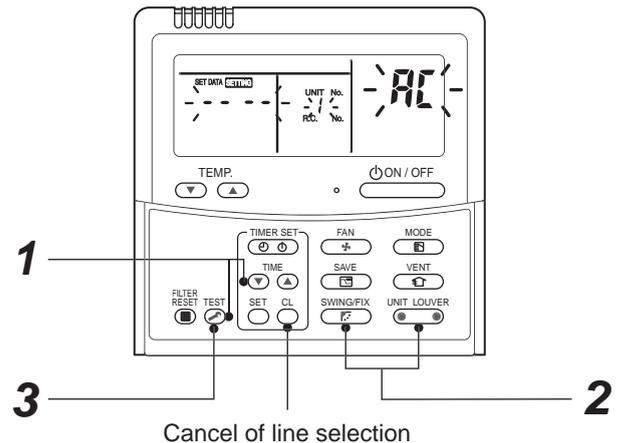
If the UNIT No. is not call up here, the outdoor unit in that line does not exist.
