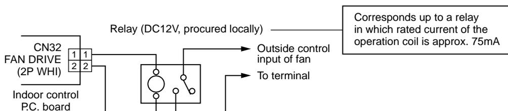
**Note)** Determine the cable length between the indoor control P.C. board and the relay within 2m.
