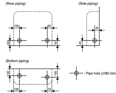
1. After determining the pipe hole position, drill the pipe hole (∅65 mm) at a slight downward slant to the outdoor side.
