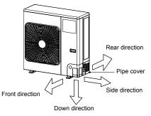
The indoor / outdoor connecting pipes can be connected in 4 directions.
