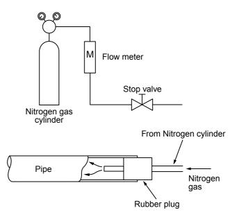
Fig. 6-5-1 Prevention of oxidation during brazing
