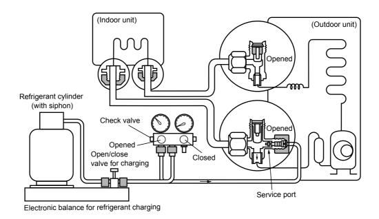
Fig. 6-4-1 Configuration of refrigerant charging
