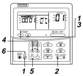
**1** Push and hold 🕅 button and "TEMP." 💌 button simultaneously for 4 seconds or more. After a while, the display flashes as shown in the figure. Confirm that the CODE No. is [01].
