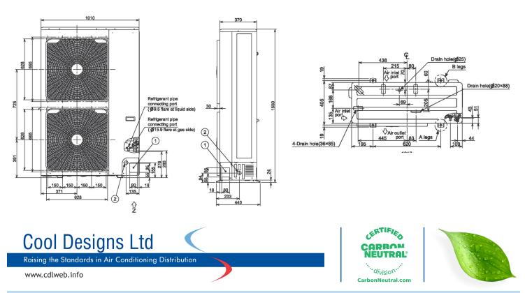
All UK duties are based on Cooling Indoor air temperature 22°C DB/16°C WB Outdoor air temperature 28°C DB 50% RH, high fan speed, 5 m pipe run. Heating Indoor air temperature 20°C DB Outdoor air temperature -5°C DB 100% RH, high fan speed, 5 m pipe run. Values are based on the maximum compressor output. Data obtained from Toshiba Air Conditioning Published Data July 2018.
