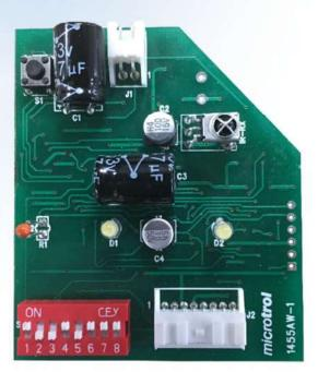
The new interface replaces the factory fitted IR Receiver PCB, referred to on the wiring diagram as "Wireless Unit Assembly, WP-033", when installed the "Mirai" unit will have local IR control as well as central control, via Toshiba's central Control Devices, BMS-CM/SM-1280## - 128 zone central remote controller, RBC-TBPTS – 64 zone colour Smart Touch Screen Central Remote, plus, many other devices.
