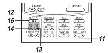
11 Used for selecting a unit while changing settings if the remote controls two or more units. UNIT button:
