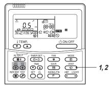
1 Push the <u>the</u> button while the system is running.
