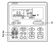
**1** Push the buttons to start operation. The operation lamp lights up.
