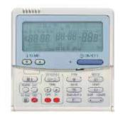
**Enter Configuration Menu** Press and hold Test(Spanner), Set & CL
