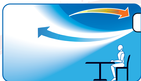
Correct louvre positioning ensures draught-free comfort
