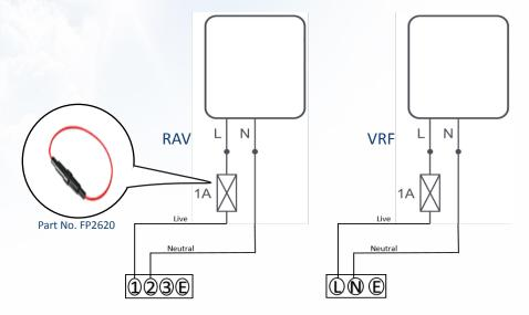
2) If your external condensate pump has a high water level switch, this can be wired into the indoor unit integrating into the installed (Where applicable) float switch
