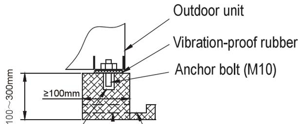
Mortar Hole (Φ100mm x Depth 150mm) Drainage (Wide 100mm x Depth 150mm)
