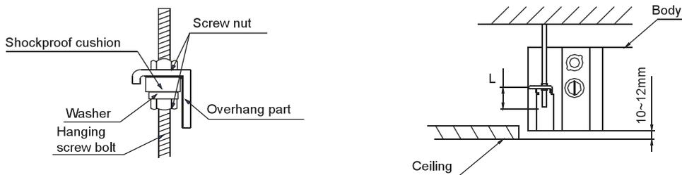
2.3.3 Screw the nuts to suspend the unit. Check the lower side of indoor unit locates at position (10 to 12mm) higher than the lower surface of the ceiling. L is about half of the screw length of the installation hook.
