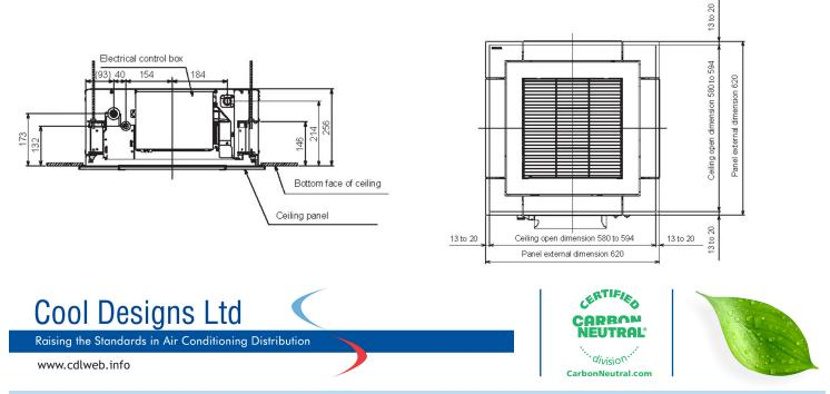
All UK duties are based on Cooling Indoor air temperature 22°C DB/16°C WB Outdoor air temperature 28°C DB 50% RH, high fan speed, 5 m pipe run. Heating Indoor air temperature 20°C DB Outdoor air temperature -5°C DB 100% RH, high fan speed, 5 m pipe run. Values are based on the maximum compressor output. Data obtained from Toshiba Air Conditioning Published Data September 2014.
