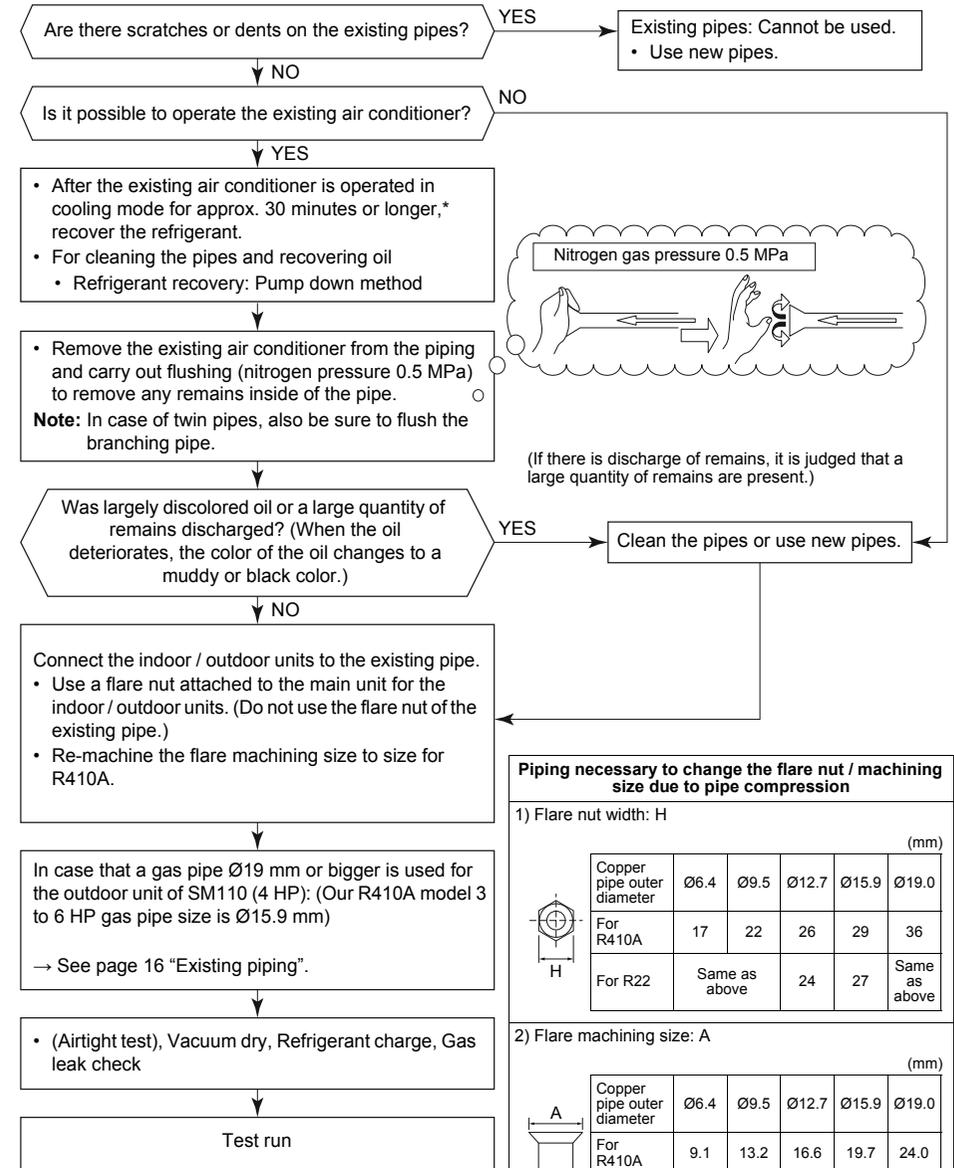
**Piping necessary to change the flare nut / machining size due to pipe compression**
