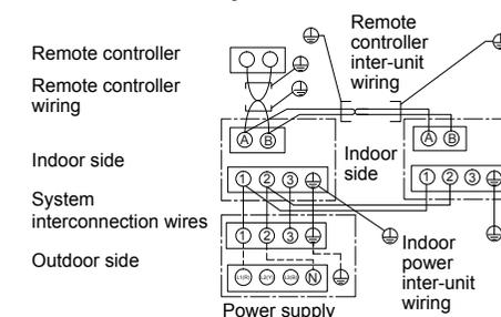
\* Use 2-core shield wire (MVVS 0.5 to 2.0 mm<sup>2</sup> or more) for the remote controller wiring in the simultaneous twin system to prevent noise problems. Be sure to connect both ends of the shield wire to earth leads.
