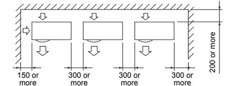
The height of the obstacle should be lower than the height of the outdoor unit.
