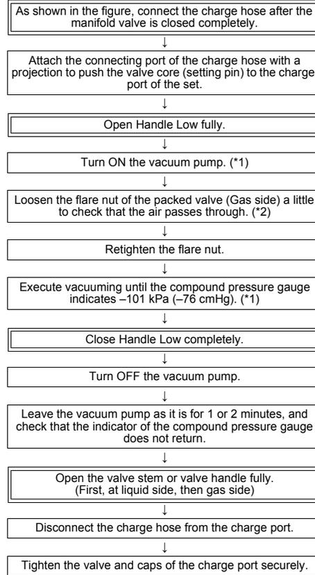
\*1: Use the vacuum pump, vacuum pump adapter, and gauge manifold correctly referring to the manuals supplied with each tool before using them. Check that the vacuum pump oil is filled up to the specified line of the oil gauge.
