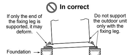
Set the out margin of the anchor bolt to 15 mm or less.
