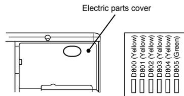
Inspection window through which to check the LED displays
