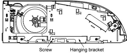
**2** Loosen the bolts fastening hanging bracket onto the indoor unit and remove the hanging bracket.
