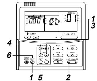
**1** Push and hold **TEST** button and **"TEMP."** button simultaneously for at least 4 seconds. After a while, the display flashes as shown in the figure. Confirm that the CODE No. is [01].
