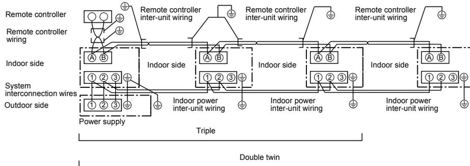
\* Use 2-core shield wire (MVVS 0.5 to 2.0 mm<sup>2</sup> or more) for the remote controller wiring in the simultaneous twin, simultaneous triple and simultaneous double twin systems to prevent noise problems. Connect both ends of the shield wire to earth leads.
