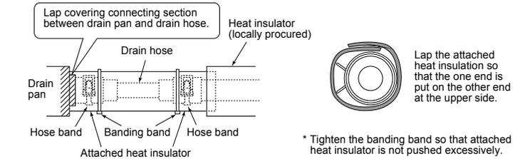
\* Fasten the binding bands in such a manner as to not squeeze the attached insulating material excessively.
