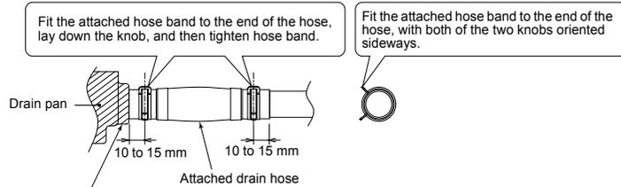
Confirm that soft hose is pushed in up to the end of the drain pan.
