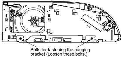
**3** Adjust the length of the two bolts for fastening the hanging bracket, as shown below.
