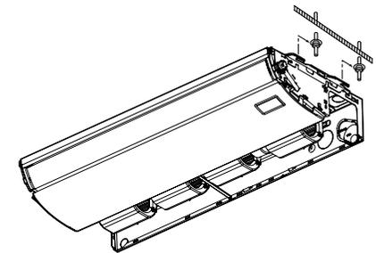
3 As shown in the figure below, fix the ceiling material securely with the double nuts.
