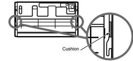
Cushions are inserted between the side panel and hanging hook for transportation. (In the two places shown above) Remove them before installation.
