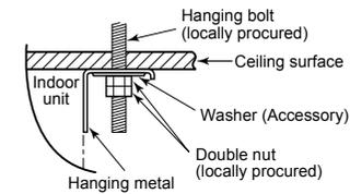
• Fix the hanging bracket as shown below if the ceiling is bent upwards when you fasten lower nuts to the hanging bracket.
