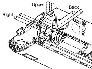
\* When Drain Pump Kit (sold separately) is installed, a refrigerant pipe can only be taken out from upper direction.
