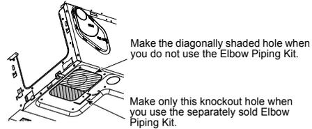
After piping, cut off the attached heat insulator of the top plate to pipe shape, and then seal the knockout hole.
