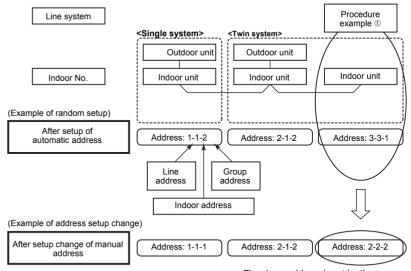
The above address is set by the automatic addressing when the power is turned on. However, line addresses and indoor addresses are set randomly. For this reason, change the setting to match line addresses with indoor addresses.
