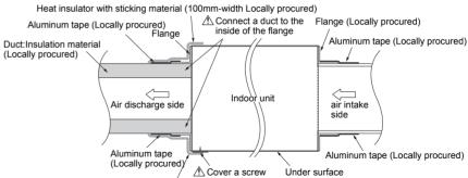
Heat insulator with sticking material (100mm-width Locally procured)
