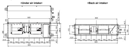
Be sure to mount an air filter to the air intake side; otherwise decrease of capacity and etc. may be caused.
