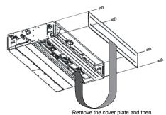
Remove the cover plate and th fix it to the bottom surface.
