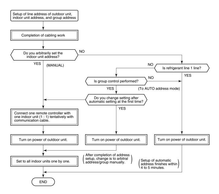
• When the following addresses are not stored in the neutral memory (IC503) on the indoor P.C. board, a test run operation cannot be performed. (Unfixed data at shipment from factory)
