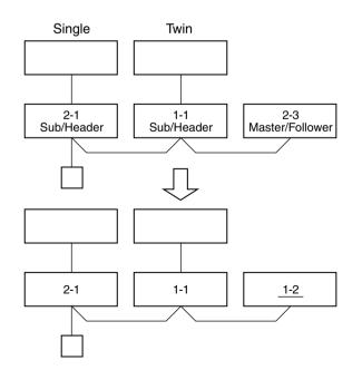
Change is necessary Manually change addresses of the multiple follower units simultaneously from the remote controller.
