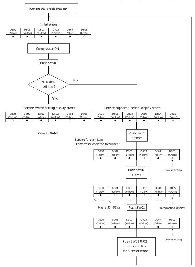
○:ON, ●:OFF, ◎:Rapid Flashing(5 times/sec), ◇:Slow Flashing(1 time/sec)
