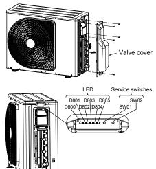
3. Turn on the circuit breaker to supply electricity. In the initial LED display status, D805 is lighted as below.
