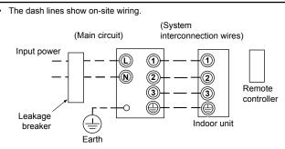
Connect the indoor/outdoor connecting cables to the identical terminal numbers on the terminal block of each unit.
