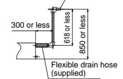
Drain up setup dimensions
