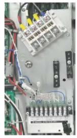
close-up view of terminal block sub-assembly
