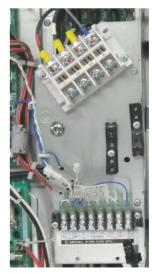
Close-up view of terminal block sub-assembly
