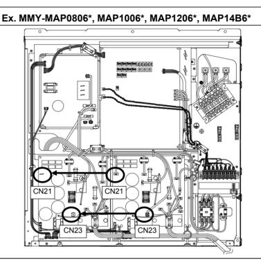
Change the connection of wiring which is connected to the CN21, 23 of Comp-IPDU2 • Change to CN21 of Comp-IPDU1 from CN21 of Comp-IPDU2 • Change to CN23 of Comp-IPDU2 from CN23 of Comp-IPDU2
